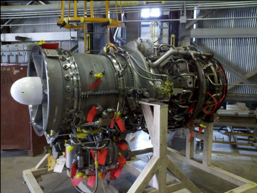
GE LM-1600 Gas Turbine (15 MW Capable)
